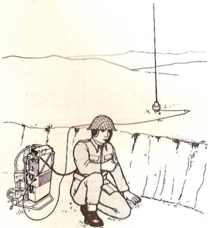
Fig.20 UK/PRC-352 used with Ground-Spike Antenna
